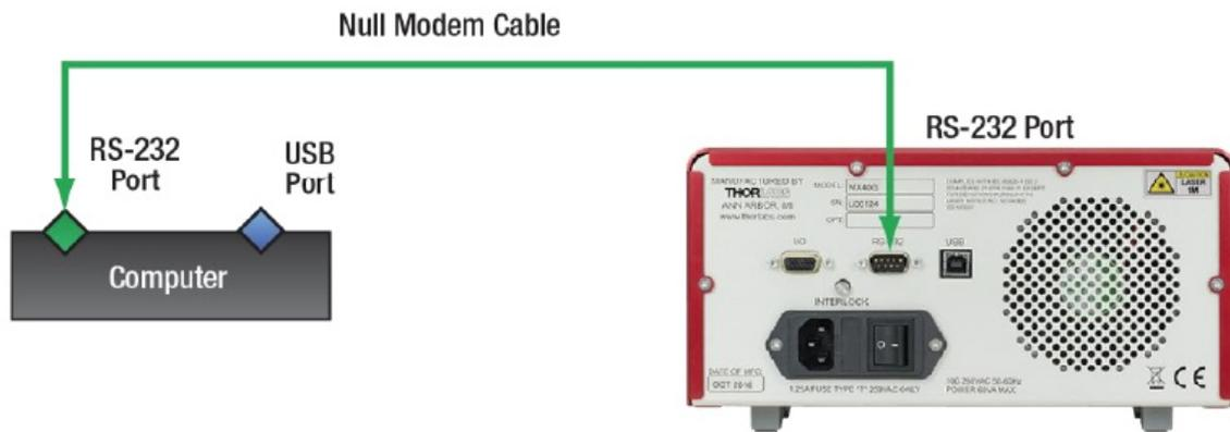
**Figure 4** Connecting the Computer and MX / MBX / TLX1 / TLX2 Series Instrument via the RS-232 Ports
