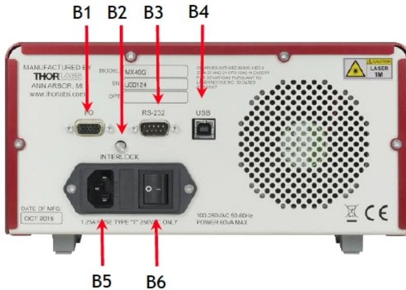
**Figure 1 Back Panel of the MX40G**
